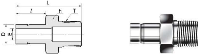
Connects fractional S-LOK port to female NPT thread
