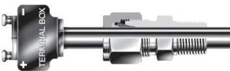
S-LOK thermocouple connector has no shoulder nor sizing angle inside the fitting; the features enable thermocouple to go through the fitting's thread end.
