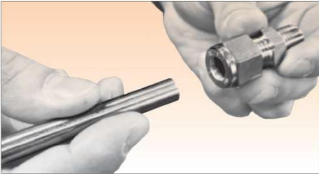
Mark the nut at the 6 o'clock position before placing the spanner.
