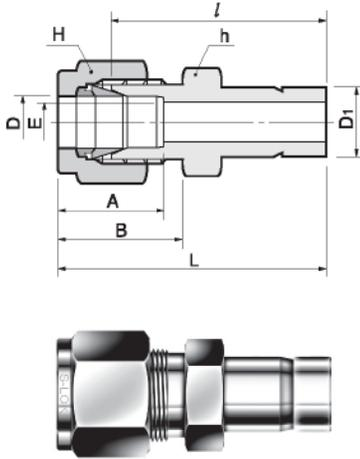
Connects metric tube to fractional S-LOK port
