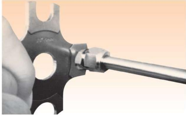
Gap Inspection Gage assures the installer or the inspector that the instrument has been sufficiently tightened during the first installation inspection.
