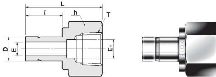
Connects fractional S-LOK port to male ISO tapered thread
