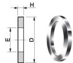
A gasket is dropped into the flat bottom of the female thread. The face of the male thread exerts a load on the gasket to seal.
