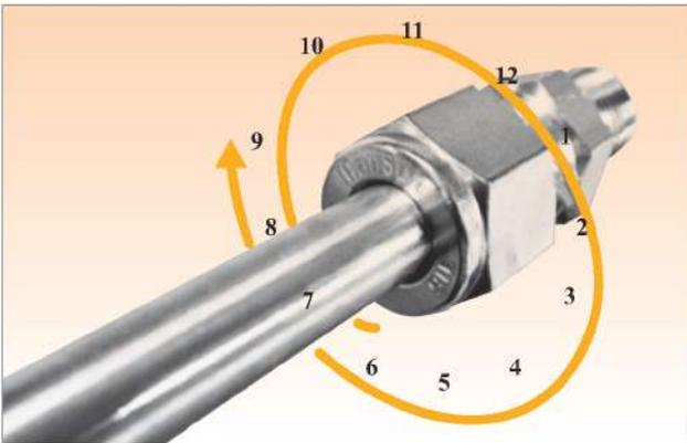
While holding the fitting body steady, tight the nut with the spanner by turning one and one-quarter (1 1/4) clockwise. Make sure that the spanner's starting point at 6 o'clock is being positioned at 9 o'clock after tightening 1 1/4 clockwise.
