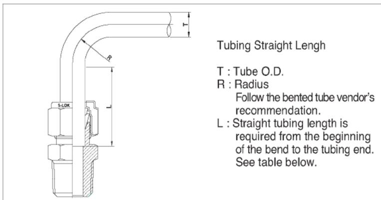
• Length of straight section of Fractional tubing Unit:Inch
