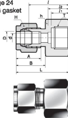
Connects metric tube to ISO parallel thread (gauge)
