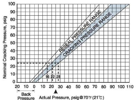
**Note** -When the check valve is not actuated for a period of time, it may require initially crack at higher than the above cracking pressure ranges.
